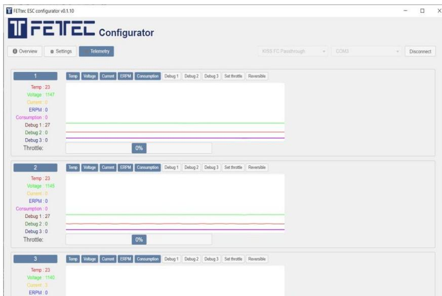
In **Telemetry** page you can spin the motors, view and debug the Motor telemetry.
